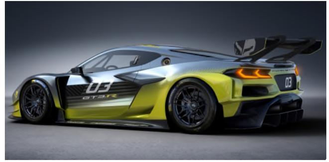
The Corvette Z06 GT3.R is closely related to the street-going C8 Corvette Z06, with both machines sharing the same aluminum chassis and naturally aspirated 5.5L V8 LT6 engine, plus similar aerodynamic features as well. Of course, the racing machine is also extensively modified for competition use. Notably, the majority of Corvette's rivals already offer a customer GT3 race car for purchase, including Audi, BMW, Ferrari, Lamborghini, Porsche, and others.
